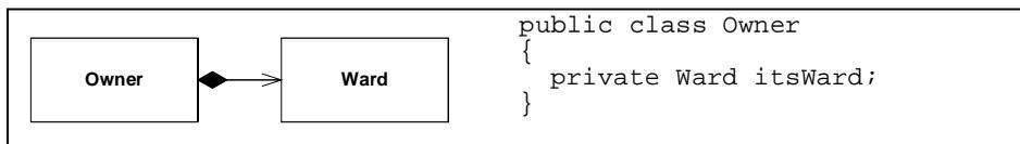
The same rule applies to Composition that applied to aggregation. There can be no cycles of instances. An owner cannot be its own ward. However UML provides quite a bit more definition.
