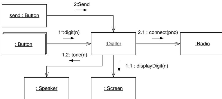
Once the connection has been established, the `Radio` can tell the `Screen` to light up the “in use” indicator. This message will almost certainly be sent in a different thread of control (which is denoted by the letter in front of the sequence number). The final collaboration diagram is shown in Figure 2-6.
